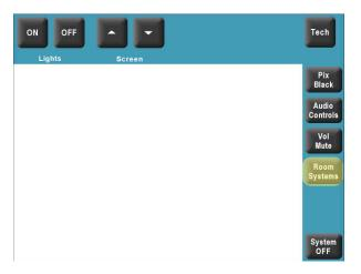
The System Off button turns off the Smart Desk. The process for turning off the Smart Desk will be discussed later.
